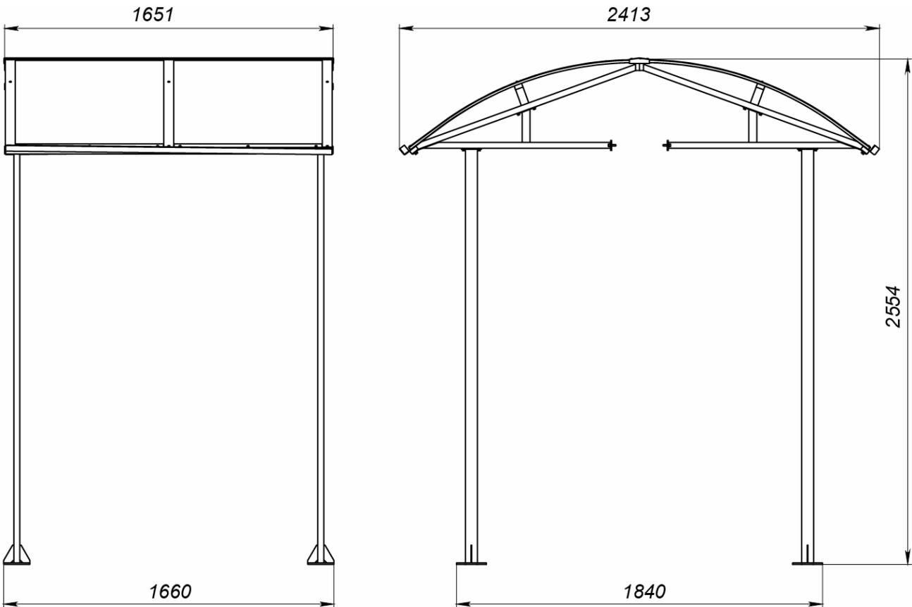
Figure 1. Overall dimensions of the canopy
