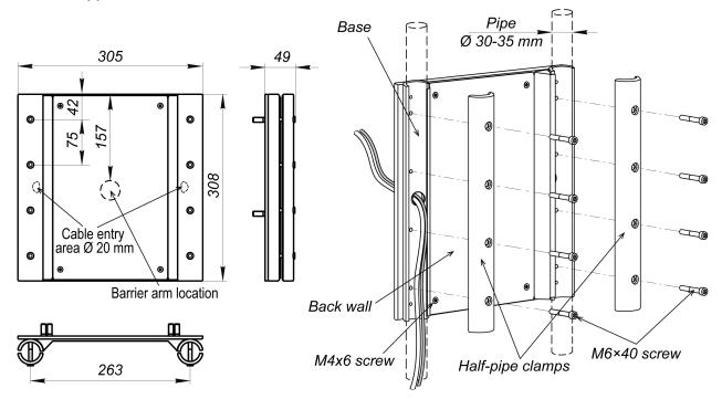
Figure 17. Dimensions and installation procedure for the MT10.1 mounting bracket
