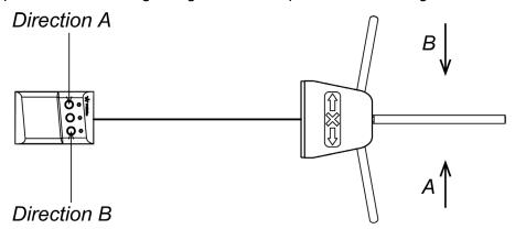
Figure 13. Standard RC-panel orientation regarding the turnstile post
