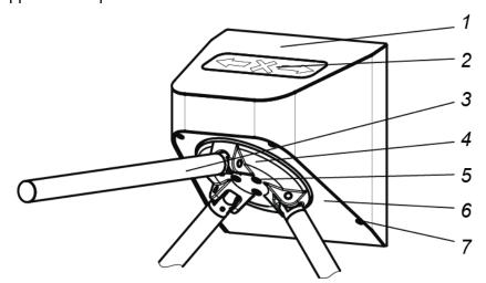
Figure 5. Turnstile components without a mounting bracket (post)
