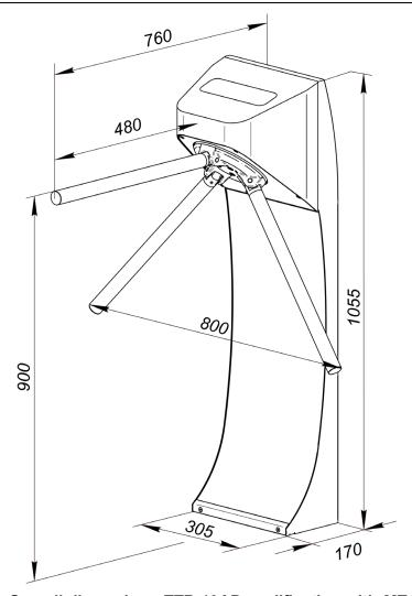
Figure 4. Overall dimensions TTR-10AB modification with MT10.3 post
