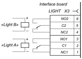
Figure 15. Light A and Light B pass elements
