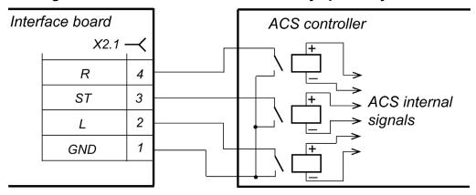
Figure 12. ACS control elements – scheme with an open collector output
